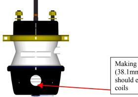
Making the 1.5"-2.5" (38.1mm – 63.5mm) cut should expose spring coils
