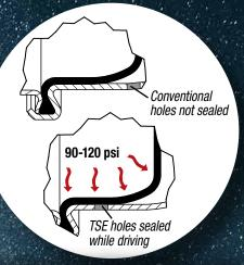
Proprietary TSE Sealed When It Counts<sup>™</sup> utilizes air pressure in chamber to push the diaphragm against the housing drain holes to create a secure seal against moisture and contaminates while driving. When parked, drain holes open up to allow draining and ventilation.
