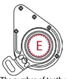
The number of teeth on the worm wheel which mates with the camshaft can be counted (E).
