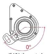
If ASA the control arm angle can be checked. For S-ASA this is not applicable.
