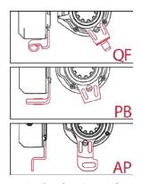
On both ASA and S-ASA the Anchor Point type will be Quick-Fit, Peg Bolt, or Anchor Pin (D).
