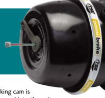
Pneumatically cage the unit by putting system air to the parking system. This will push the spring pressure plate to the rear of the housing.
